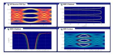
A key feature of the PAM-4 tool is to optimize the eye center reflecting a receiver with maximum horizontal and vertical margins. You have the option to lock the vertical slicer to a single phase for all three eyes.
