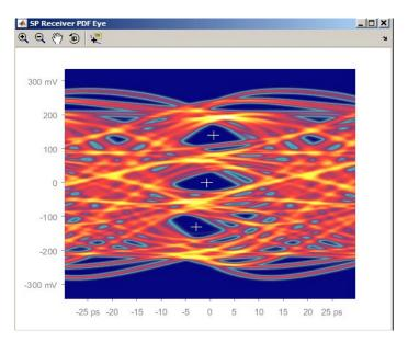
The PAM-4 analysis has full signal path emulation tools that support Continuous Time Linear Equalizer (CTLE), channel emulators described by S-parameters or TDR waveforms, and receiver equalizers Feed Forward (FFE) and Decision Feedback (DFE).
