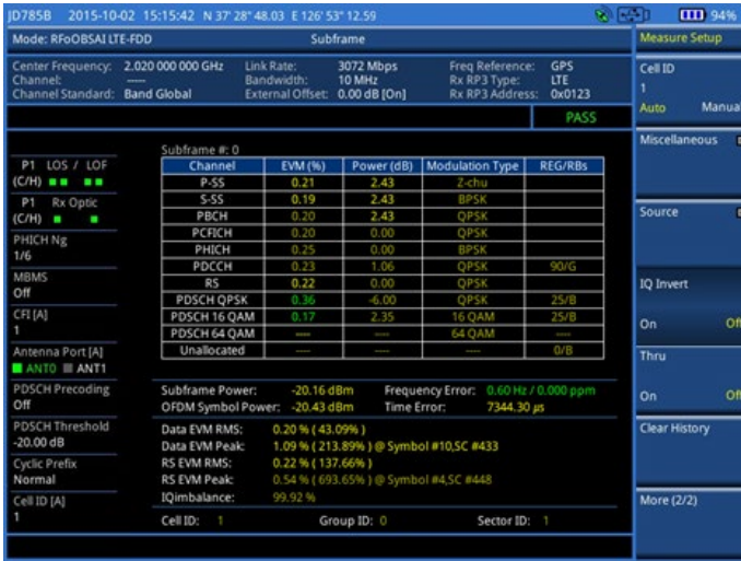
RfOBSAI LTE-FDD signal analyzer window
