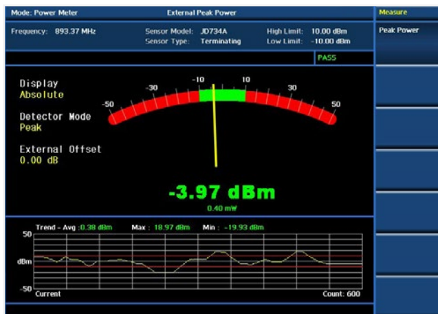
Power meter test (RF or optical)
