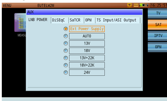
Figure 6-59 LNB Power Supply Control
