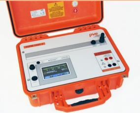
that the measured I-V-curves permit further explanations about the electrical characteristics of the verified module or string. That is why the PVPM 1500X is suitable as an instrument in research and for development purposes as well.
