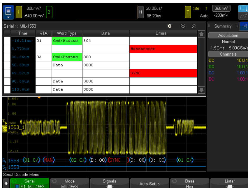
Figure 2. MIL-STD 1553 decode on an InfiniiVision X-Series oscilloscope.
