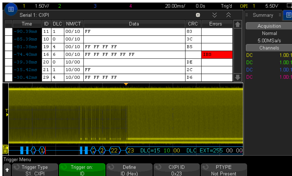
Figure 8. CXPI decode on an InfiniiVision X-Series oscilloscope.
