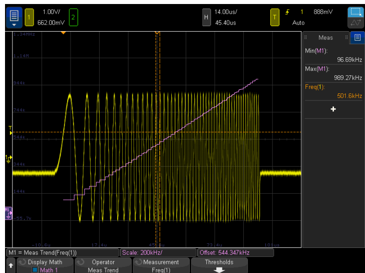
Figure 10. Measurement trend math function used to plot frequency versus time of a FM burst.
