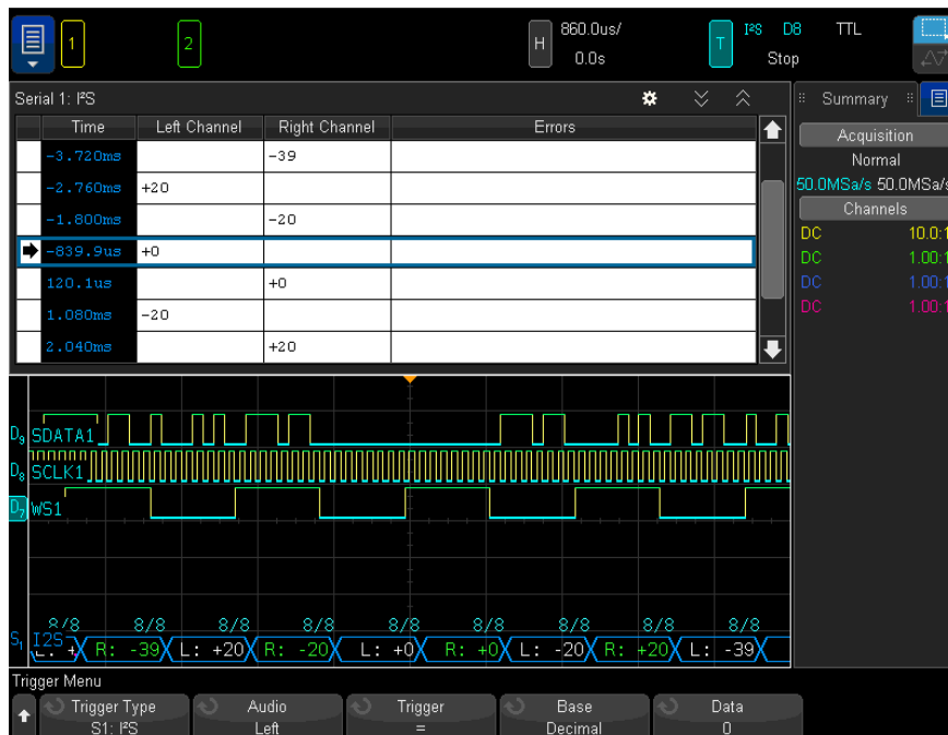
Figure 5. I 2 S decode on an InfiniiVision X-Series oscilloscope.
