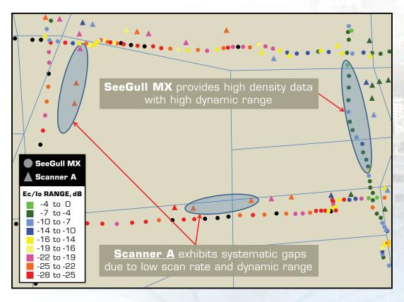
This drive test plot shows SeeGull MX with high data rates and dynamic range alongside Scanner A with lower data rates and dynamic range. The data from SeeGull MX provides more information about the network and increases the confidence level of the collected data.
