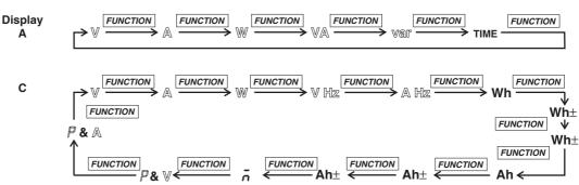
Wh $\pm$  and Ah $\pm$  will light twice.  $\bar{n}$  and  $\bar{P}$  are displayed on the top of display C. You can reverse the order by first pressing the SHIFT key followed by the FUNCTION key.
