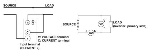
Wiring Example of a Current Measurement Circuit
