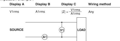
$\mathcal{F}_{-b}$ : Displays the result of display A ÷ display B.
