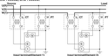
Wiring example of a three-phase, four-wire system (3P4W) when using a PT/CT... Can be applied to model 760503.
