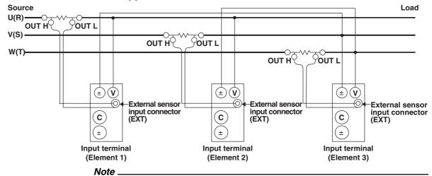
In 3P3W and 3V3A systems, the wiring system may be different between the WT210/230 and another product (another digital power meter) due to the differences in the input element that is wired. To achieve correct measurements, check the wiring system.
