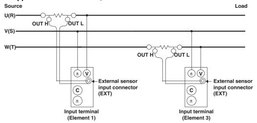
Wiring example of a three-phase, four-wire system (3P4W) when using an external shunt ... Can be applied to model 760503.
