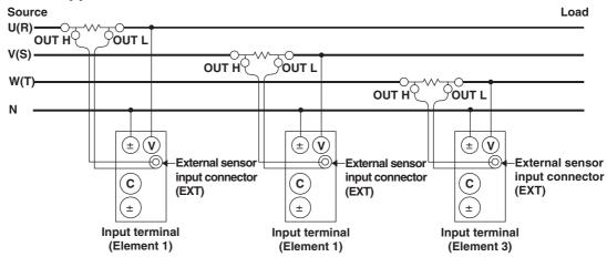
Wiring example of a three-voltage, three-current system (3V3A) when using an external shunt ... Can be applied to model 760503.
