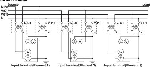
Wiring example of a three-voltage, three-current system (3V3A) when using a PT/CT ... Can be applied to model 760503.
