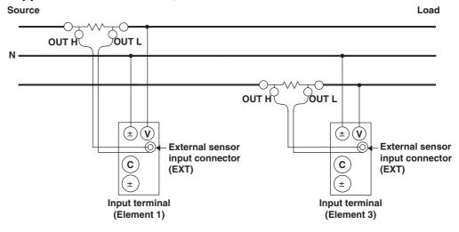
Wiring example of a three-phase, three-wire system (3P3W) when using an external shunt ... Can be applied to models 760502, and 760503.
