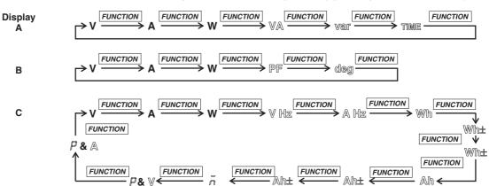
Wh $\pm$  and Ah $\pm$  will light twice.  $\bar{n}$  and  $\bar{P}$  are displayed on the top of display C. You can reverse the order by first pressing the SHIFT key followed by the FUNCTION key.
