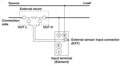
Wiring example of a single-phase, three-wire system (1P3W) when using an external shunt ... Can be applied to models 760502, and 760503.
