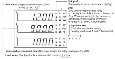
\* The limit values on display A and B will show the pairs of ch1&ch2 and ch3&ch4 alternately by pressing the \bigvery \bigvery \bigvery \bigvery \lambda keys. Check the displayed limit value, unit, or the limit value setting menu to see which pair is being displayed,
