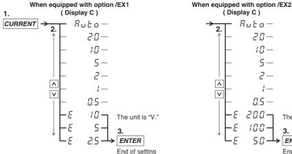
(Display C) Ruto-20-٨  $\overline{\mathsf{v}}$  $\Pi S -$ 200 The unit is "mV." 100 **ENTER** End of setting
