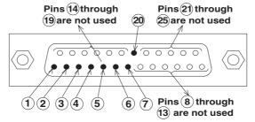
SERIAL Connector: DBSP-JB25S or equivalent
