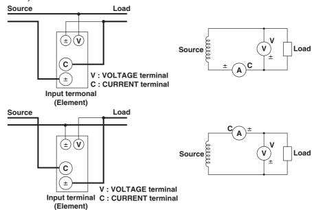
Wiring example of a single-phase, three-wire system (1P3W) ... Can be applied to models 760502, and 760503.
