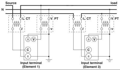
Wiring example of a three-phase, three-wire system (3P3W) when using a PT/CT... Can be applied to models 760502, and 760503.
