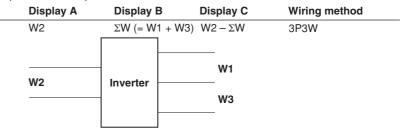
$\mathbb{R}_{11}$  b: Displays the result of display A  $\times$  display B.
