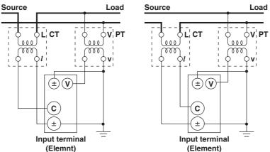
Wiring example of a single-phase, three-wire system (1P3W) when using a PT/CT... Can be applied to models 760502, and 760503.
