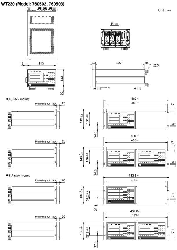
Unless other wise specified, tolerance is  $\pm 3\%$  (However, tolerance is  $\pm 0.3$ mm when below 10mm)
