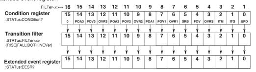
The meaning of each bit of the condition register is as follows.
