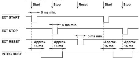
As shown in the timing chart, the **INTEG BUSY** output signal level goes low while integration is in progress. The signal can be used to monitor integration, etc.
