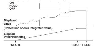
Even when stopping integration while the hold function is on, the displayed integrated
