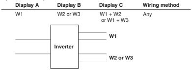
$\overline{A}$  - b: Displays the result of display A – display B.
