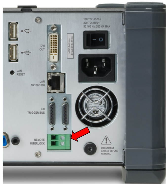
Figure 2: Remote Interlock Terminal
