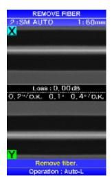
Splice loss may be improved in some cases by additional arc discharges. Press <u>SET</u> key for an additional arc discharge (re-arc). Splice loss estimate and splice check are performed again.
