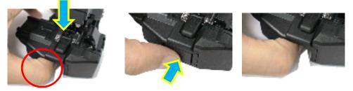
Press down the cutting lever. Release the pressure on the cutting lever. A spring force will bring it to its open position.
