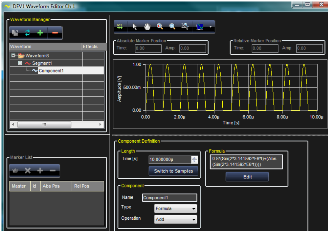
Figure 3-18. A half-wave rectified sine waveform. The actual formula used here is 0.5*(\sin(2*3.141592*E6*t)+(\text{Abs}(\sin(2*3.141592*E6*t)))) . Set the time to 10.000000\mu to view the graph as previously shown.
