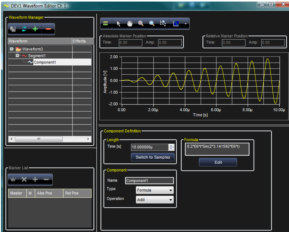
Figure 3-10. A linear amplitude sweep of a 1 MHz sine waveform. The actual formula used here is 0.2 \cdot E6 \cdot t \cdot \sin(2 \cdot 3.141592 \cdot E6 \cdot t) . Set the time to 10.000000\mu to view the graph as previously shown.
