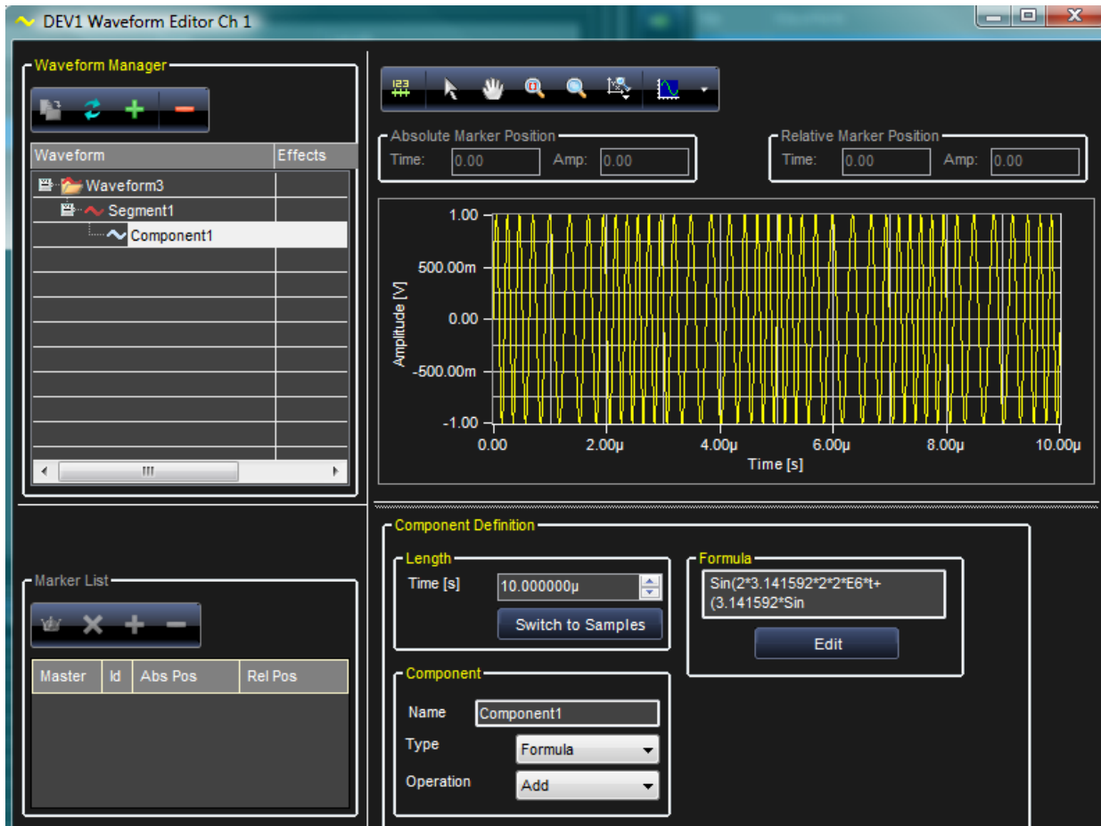
Figure 3-12. A phase modulation waveform. The actual formula used here is \text{Sin}(2*3.141592*2*2*E6*t+(3.141592*\text{Sin}(2*3.141592*0.4*E6*t))) . Set the time to 10.000000µ to view the graph as previously shown.
