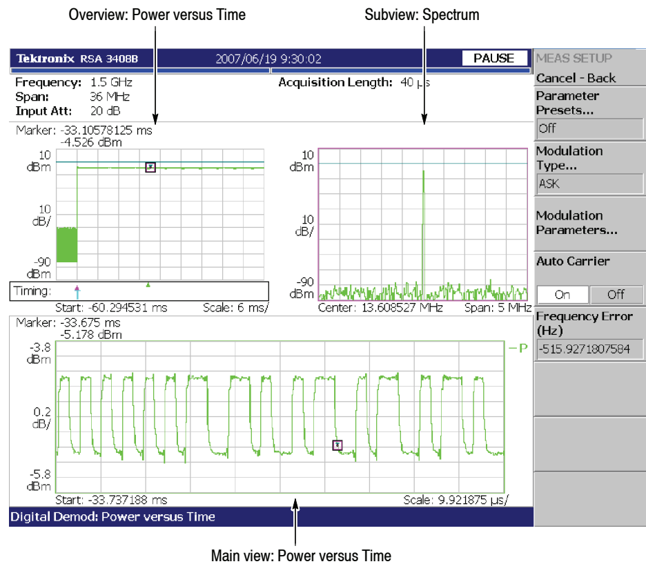
Figure 3-48: Power variance measurement
