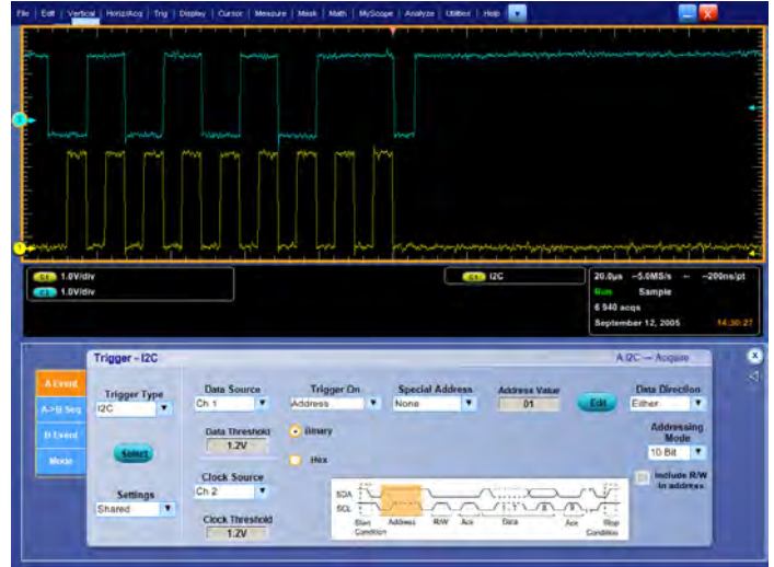
Easily trigger on a specific I2C address.
