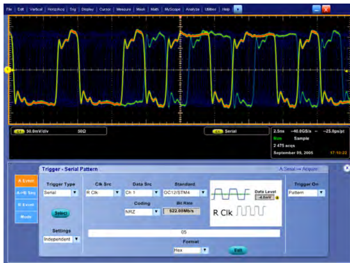
Serial pattern triggering to debug pattern-dependent issues.
