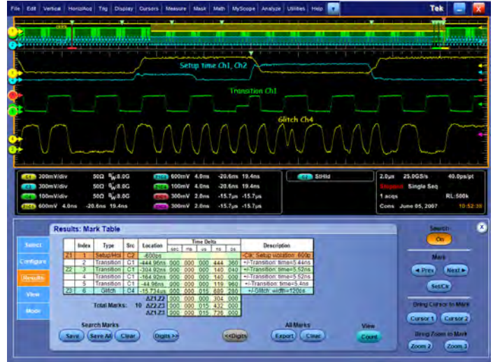
Accelerating the research of specific events in an acquired waveform.
