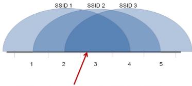
SSID 2 experiences interference from SSID 1 and SSID 3
