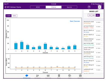
The **Utilization** graph in the top pane shows the channel utilization for all channels in the selected band. Touching a bar within the graph highlights the bar for that channel (the blue bar will turn green) and the "BSSID List" changes to the Channel Summary which includes values associated with that particular channel.
