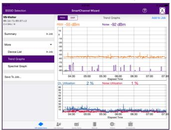
The utilization graph shows both the Channel Utilization (blue line) and the actual utilization due to noise (red line).
