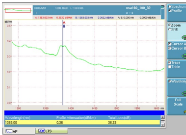
An attenuation profile showing a loss vs. wavelength measurement
