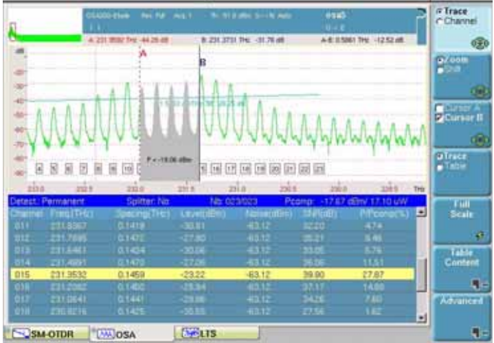
Fig. 44 Display of total power, gain tilt and slope of the gain between the cursors
