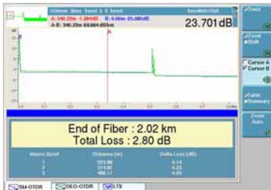
Fig. 34 Fault location Bend.
