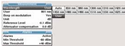
Fig. 87 Configuration of power measurement
