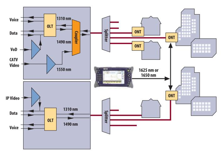
The LM OTDR performs in-service measurements
