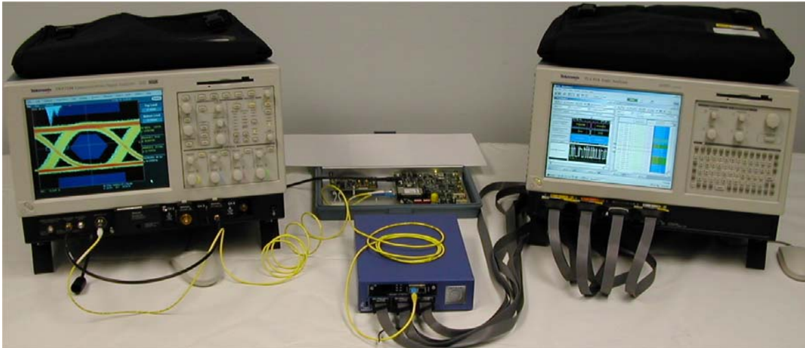
Singulus being used to excite DUT with Tektronix scope and Logic Analyzer measuring the results
