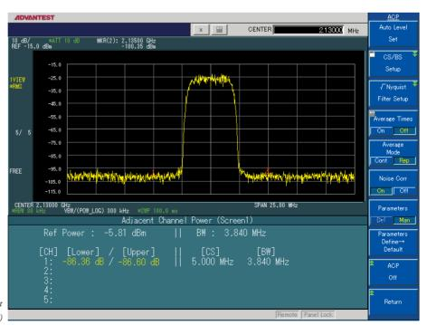
3GPP 1-carrier/ACLR measurement (noise correction enabled)
