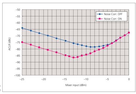
Dynamic range of ACLR measurement at the mixer input level
