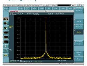
Noise/1 Hz: -123 dBc/Hz (20-kHz offset) @ 800 MHz
