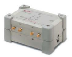
The high-impedance differential IQ signal converter circuit, which is independent from the R3671/3681 signal analyzer, can be placed close to the target device. The high-impedance signal line between a DUT and the measuring device can thus be shortened, and this reduces adverse effects on modulation precision by stray capacitance on the signal line and differences in line length.
