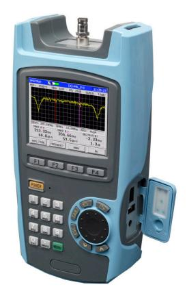
The DTVLINK-C measures a comprehensive set of digital signal parameters (Channel Power, MER, BER, Constellation Diagram), as well as analog signal performance characteristics (Single-Frequency Level, Scan, Tilt, HUM, C/N, Depth of Modulation), and Spectrum Analysis. In Level and Fast Spectrum Modes, the Peak-Hold function detects intermittent interference as a troublshooting aid useful in HFC network construction and maintenance.
