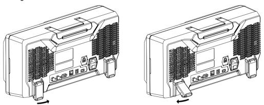
Figure 1-4 To Adjust the Supporting Legs
