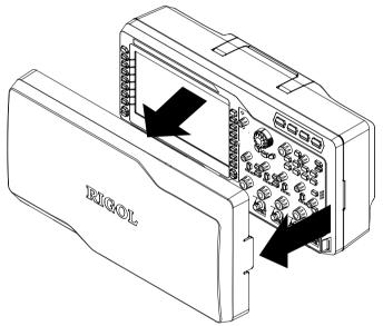
Figure 1-3 To Remove the Cover
