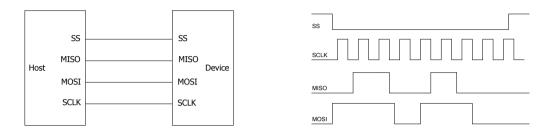
**SS:** set the polarity to "Low" or "High". When SS selection is valid, the SPI bus samples data from MISO and MOSI at the jumping point of SCLK.
