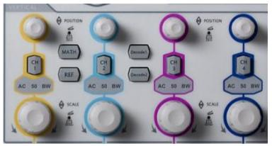
• **CH1**, **CH2**, **CH3**, **CH4**: analog input channels. The four channels are marked by different colors which are also used to mark both the corresponding waveforms on the screen and the channel input connectors. Press any key to open the corresponding channel menu and press again to turn off the channel. AC: illuminated when AC channel coupling is enabled.
