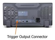
Press **Utility**  $\rightarrow$  **Aux Output** to select "TrigOut". When the oscilloscope is triggered, it will output a trigger signal determined by the current trigger setting through the **[Trig Out/Calibration]** connector.
