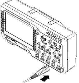
Figure 1-6 To Connect the Probe
