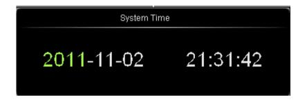
In the figure, the item in green (such as 2011) is the item that can be modified currently. Use  $\checkmark$  to modify and press down  $\checkmark$  to complete the input. The order of time modifications is: year (2011)  $\rightarrow$  month (11)  $\rightarrow$  date (02)  $\rightarrow$  hour (21)  $\rightarrow$  minute (31) $\rightarrow$  second (42). The setting range of each item conforms to the convention:
