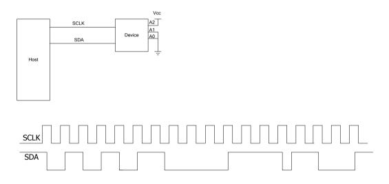
**SCLK:** sample the SDA on the clock rising edge or falling edge. **SDA:** denote the data channel.
