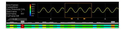
**Error Frames:** the total number of error frames discovered in this analysis. The number of error frames is related to the error frame threshold currently set.
