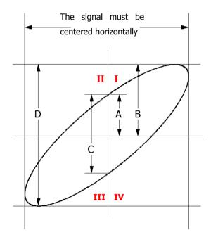
According to  $sin\theta = A/B$  or C/D (wherein,  $\theta$  is the phase deviation angle between the two channels and the definitions of A, B, C and D are as shown in the figure above), the phase deviation angle is obtained, that is:
