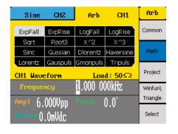
The model AD8610 have non-volatile memory to create, store, and recall up to 10 different arbitrary waveforms of up to 16,000 points each. Users can also output any of the 48 built-in predefined arbitrary waveforms.
