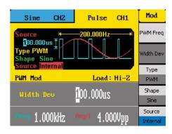
This instrument is capable of many different types of modulation for various applications. Modulate your waveforms with AM, DSB-AM, FM, PM, ASK, FSK, and PWM modulation schemes.
