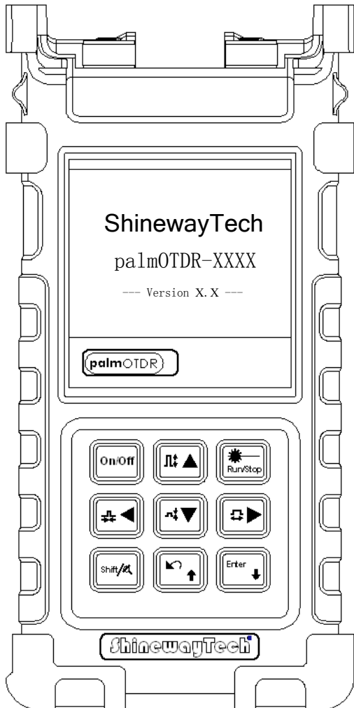
Figure 2-2. Operation Interface of AD20S OTDR
