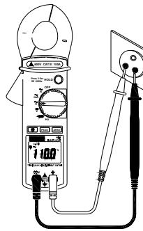
Set the switch to  $V\sim$  for an AC voltage measurement and to  $V=$  for a DC voltage measurement.
