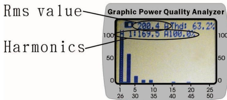
%THD-F: Total Harmonic Distortion with respect to Fundamental frequency
