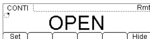
Figure 2-27 Continuity Testing Interface
