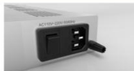
• Power supply • Power switch(left)protective tube(middle) power socket(right)
